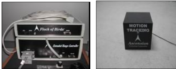
Figura 1. Sensor, controlador e transmissor do Flock of Birds .
