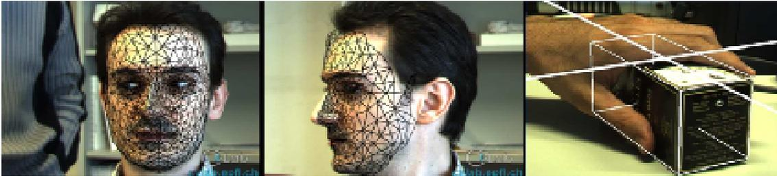
**Figure 1.13. Tracking of a human face and a tea box using an interest point based technique [Vacchetti et al 2004a].**
