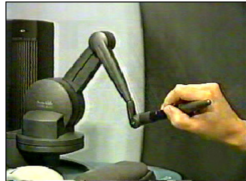
FIGURE 5. HAPTIC DEVICE FOR INTERACTION WITH TACTILE SENSATION AND FORCE FEEDBACK.
