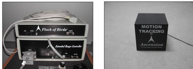
**Figura 2. Sensor, controlador e transmissor do Flock of Birds .**
