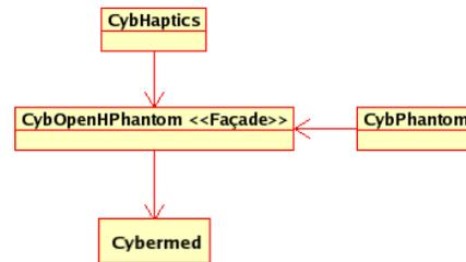
Figure 3. Classes to support Phantom devices in CybHaptics.
