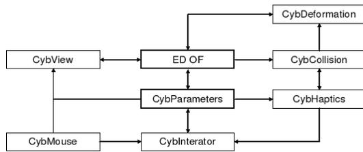
Figure 1. CybHaptics and its integration to the CyberMed system.
