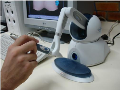
Figure 3. The haptic device Phantom Omni.
