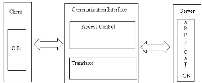
Fig. 3. Communication Interface of the Intelligent Campus.
