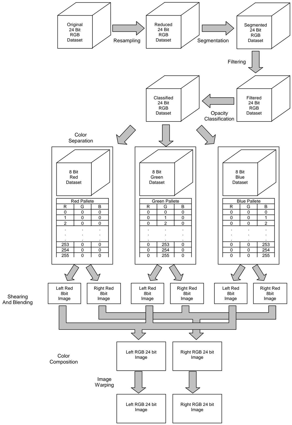
Figure 02 – The Volume Rendering Pipeline
