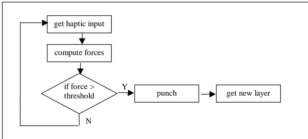
**Figure 06 - State Machine for Haptic Loop**
