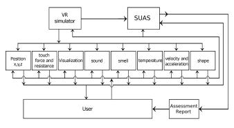
FIGURE. 1 DIAGRAM OF A VR SIMULATOR WITH A SUAS. ADAPTED FROM [13].
