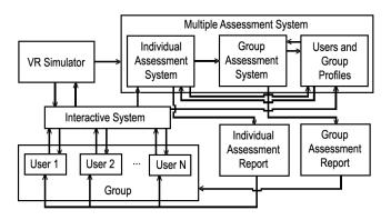
FIGURE. 3 DIAGRAM OF NEW MUAS. ADAPTED FROM [17]
