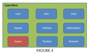
MODULES STRUCTURE OF THE CYBERMED, HIGHLIGHTING THE ASSESS MODULE RESPONSIBLE TO REALIZE USER'S ASSESSMENT. ADAPTED FROM [15].
