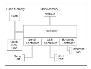
FIGURE. 3 Architecture of an embedded system. Adapted from Hallinan [16].
