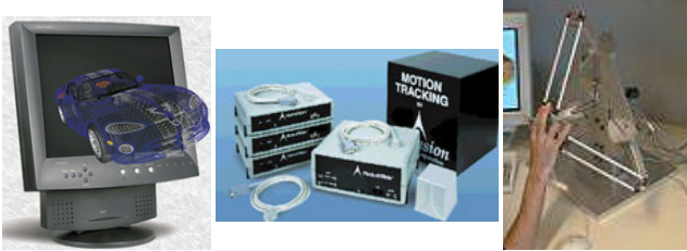
Fig. 1. Devices used to explore senses in VR systems. From left to right: auto-stereoscopic displays, motion-tracking set and haptic device.
