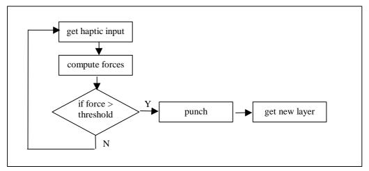
Figure 06 - State Machine for Haptic Loop
